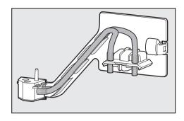
Take the cover off together with the milk pipework. Clean the whole component in the dishwasher without dismantling it.
